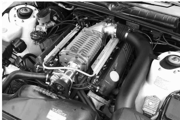
Roots charger – at engine [9]
